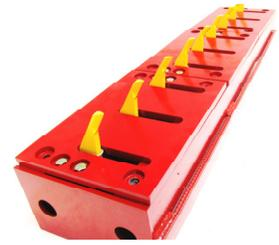
1. Install the Directional Traffic Controller perpendicular to the flow of traffic. If vehicles cross the controller at an angle other than 90 degrees the spikes may cause sidewall damage to the tires. Check all bolts to insure none have loosened during shipping, and tighten as necessary. LocTite is recommended for final installation.
