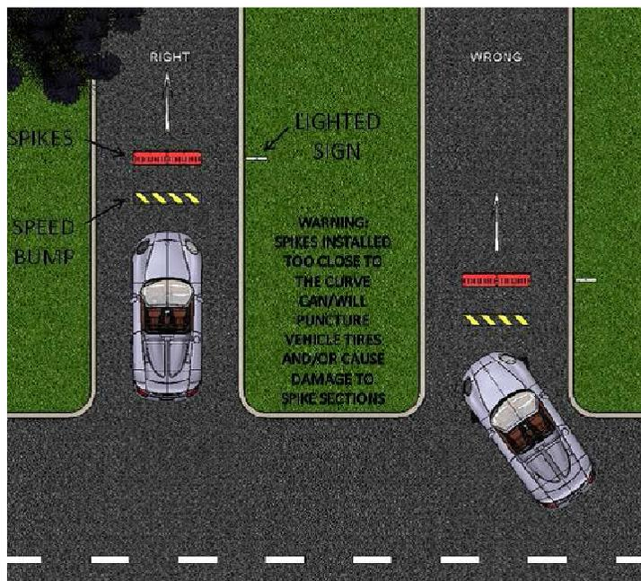
2. The maximum suggested speed vehicles may cross the controller is 5 MPH. Excessive speed will cause increased damage to the spikes and and/or broken springs will result from speed in excess of 5 MPH.
